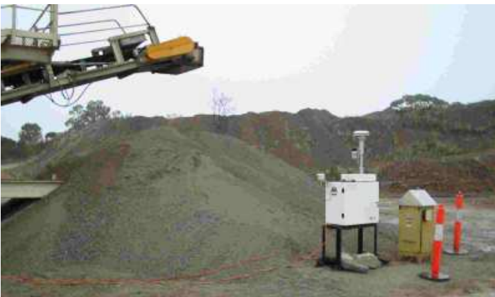
Air quality monitoring instrumentation adjacent to crushed concrete stockpile.
