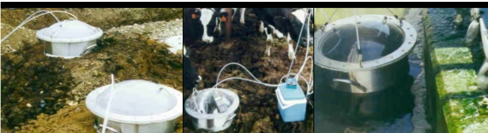
LEFT USEPA flux chamber – odour, air toxics, contaminated site
