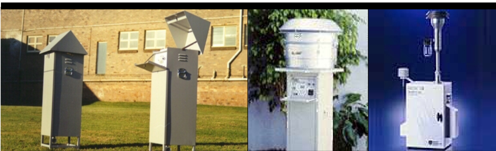
LEFT TSP sampling utilising high volume samplers
